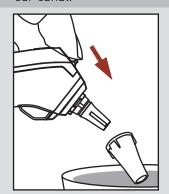
**STEP 5.** Press ejection button to discard used probe cover into clinical waste bin or recycling facitilies (in line with local guidelines).
