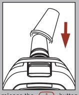
**STEP 1.** To turn on **ri**-thermo® **tymPRO**, briefly press and release the buttor ", when flashing, this indicates the **tymPRO** is ready to use and a new probe cover should be attached. Alternatively, attach a new probe cover to turn it on. When ready, the thermometer displays the last measurement.
