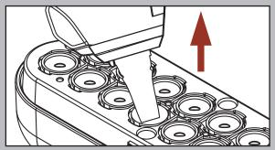
**STEP 2.** Lift the probe out of the cassette with a new probe cover attached. Do not touch the cover. Now, you can measure the temperature.
